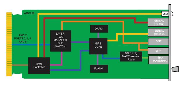
FIGURE 1. AMC228 Functional Block Diagram
